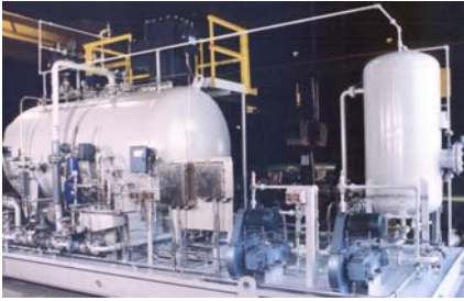
2000 bpd Crude Oil Desalter for Diesel Topping Plant British Petroleum Cusiana Field Colombia, South America
